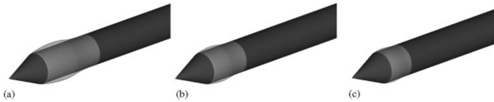
Figure 11. Cavity shapes on the wall of a conic headform/cylinder body with different cavitation indexes: (a) K = 0.30 ; (b) K = 0.40 ; and (c) K = 0.50 .
