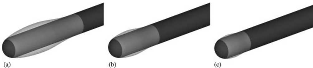
Figure 15. Cavity shapes on the wall of a hemispheric headform/cylinder body with different cavitation indexes: (a) K = 0.20 ; (b) K = 0.30 ; and (c) K = 0.40 .
